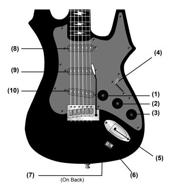
On the back panel of the guitar is the **Battery Compartment (7)**. It can be opened by pulling up the plastic cover at the finger notch. Two fresh 9V alkaline batteries should be inserted observing the correct polarity. Close the compartment. It will magnetically snap shut.
